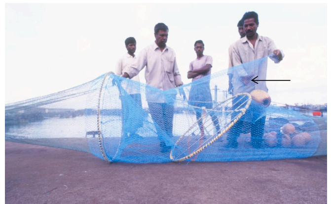
Figure 8. A TED such as this, with the escape hole arrowed, can dramatically reduce turtle mortality.
