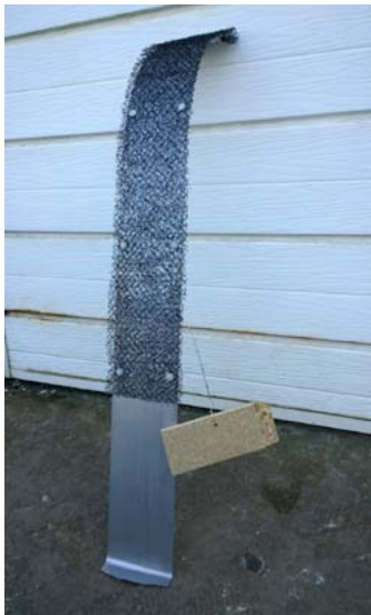
Figure 5. Ladder design to be used in continuing 2015 trials, fitted with Enkamat® and raft. Photo credit: Rose, T.
